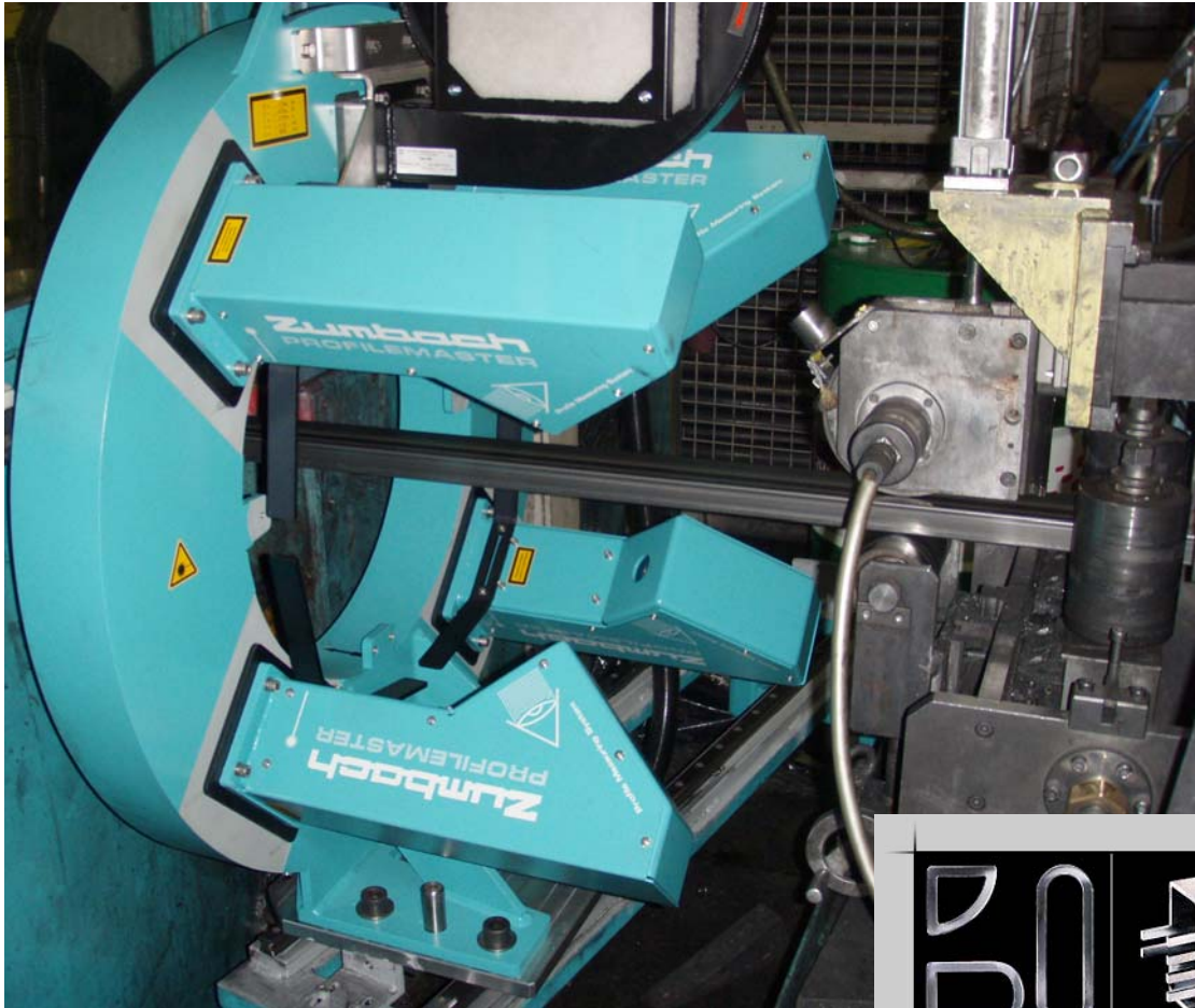
PROFILEMASTER® SPS 140-N4 Measuring System
