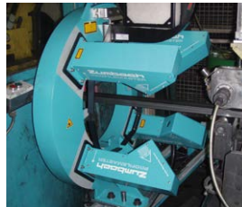
SPS 140-N4 Measurement of round and special shaped profiles.
