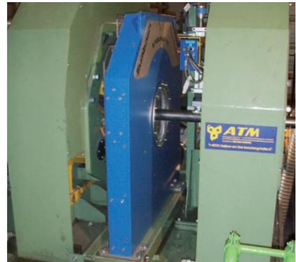
SMS 100-B6 gauge in a NDT line for cold bars
