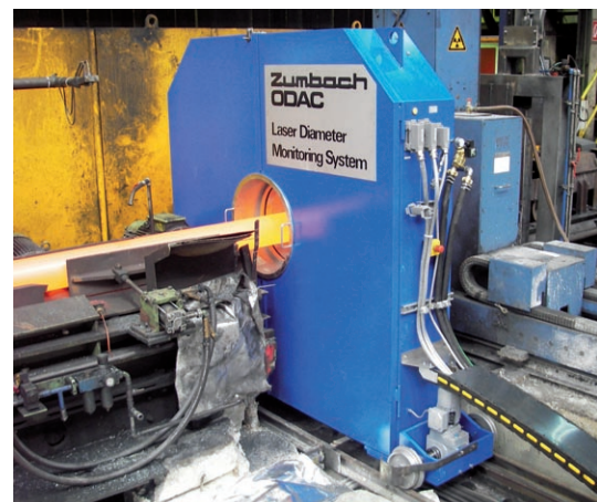
Oscillating gauge at the exit of a seamless pipe mill.
