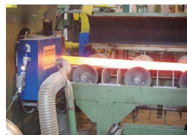
ECOGAUGE 310 in seamless tube extrusion.
