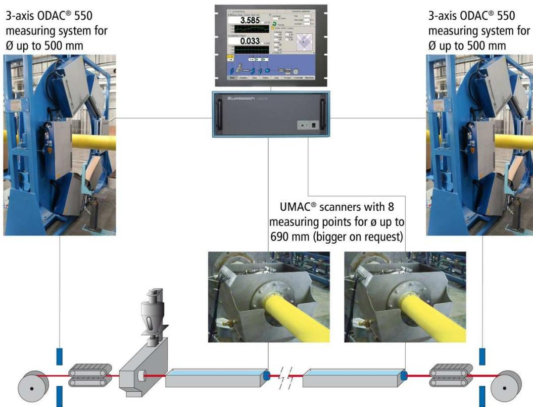
Picture: Customer specific solution with ODAC<sup>®</sup> and UMAC<sup>®</sup> gauges in an extrusion line for products up to 500mm OD.
