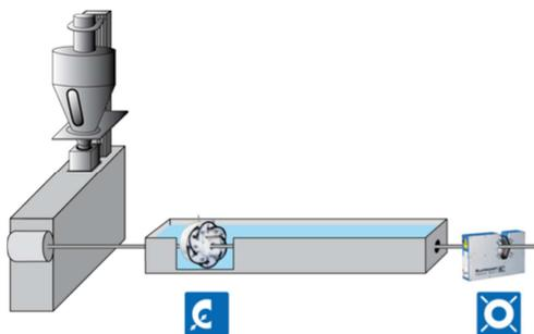
Picture: Dual Loop configuration with UMAC® at the hot end, and ODAC® at the cold.
