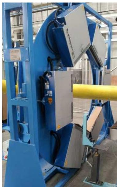
3-axis ODAC 550 system, measuring an Offshore cable of 500 mm OD
