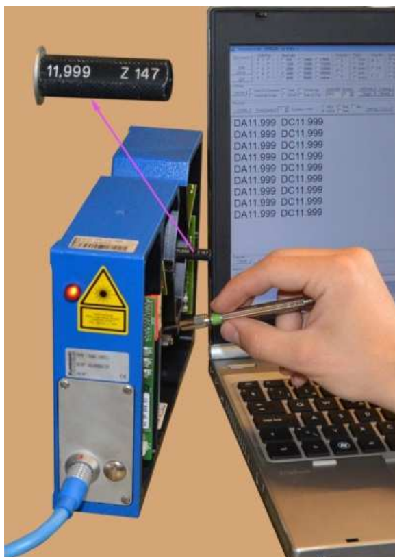
Picture: Diameter measuring head of the well known ODAC® series during calibration
